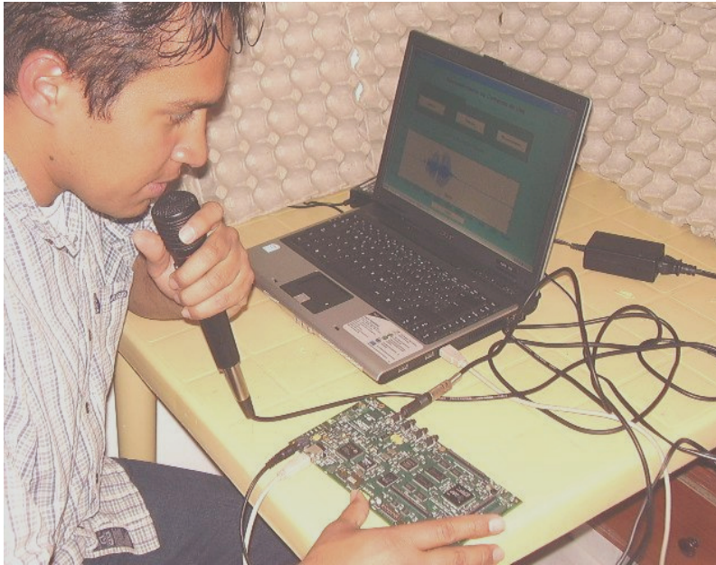
Fig. 19. ASR with the DSP Hardware (DSK6416 TI)
