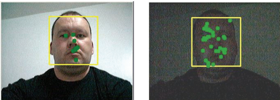
Fig. 5. The face is detected using the Haar-Classifer cascade algorithm and marked with a yellow square. Green dots mark significant features identified by the Lucas-Kanade algorithm. The image on the right demonstrates performance in poor lighting conditions.
